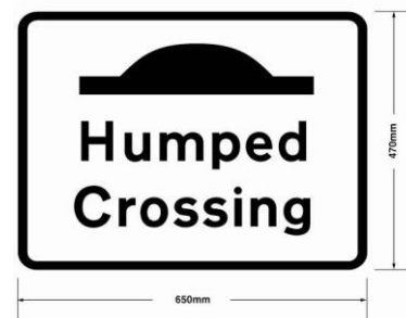
Plate for use with sign in diagram Nos. 543 or 544 in a case where a road hump is constructed and maintained in accordance with Regulation 4(4) of the Highways (Road Humps) (Jersey) Regulations 2002 547.5
